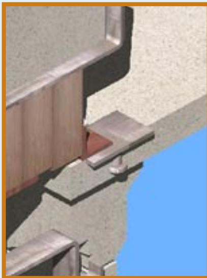
Embedded weld plate inserts support the stone structure.
