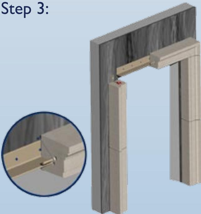
The horizontal pieces of the surround can be held in place with steel lintels and tapcon screws. Wire and pin are used to keep the stone from tipping. Drill a pin hole to secure the facing stone of the horizontal section.
