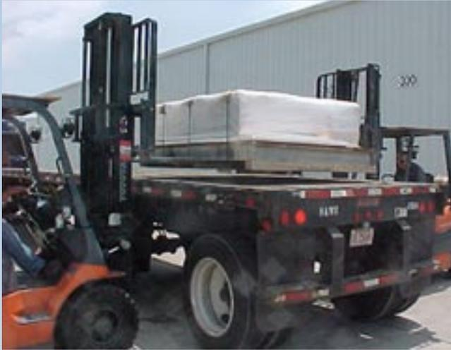
We recommend the use of two forklifts for large stone pallet removal. Adequate space around the trailer will be necessary to maneuver properly.
