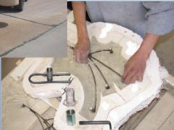
Threaded inserts can be added in the manufacturing process to attach the stone to other structures.
