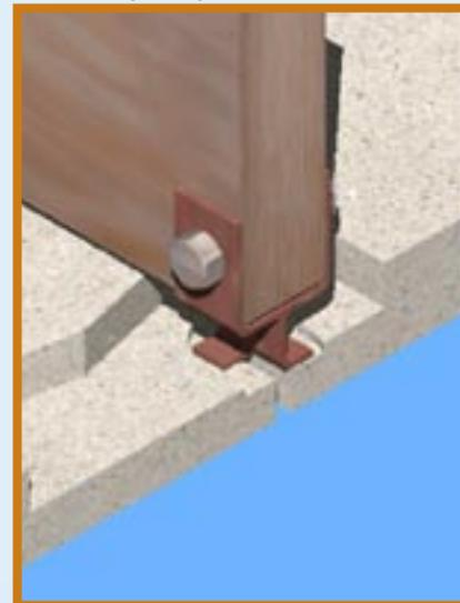
Two-Way Clips require inset grooves to protect the stone from cracking.
