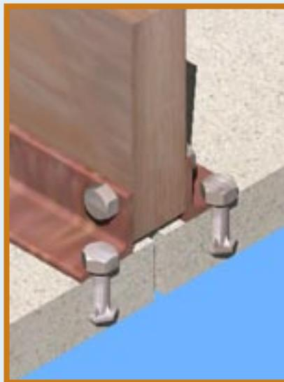
Inset threaded bolts fasten onto a locking plate.
